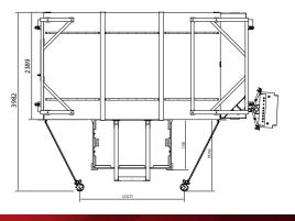
The **PRO FI** is designed for rapid inspection of small to large sized casting parts. The flexible part table allows the inspection of several smaller parts at the same time or the inspection of a single casting. Versatile manipulator enables easy program creation without programming knowledge.
